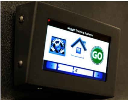
The XCT is a non-turning target retriever operated by a touchscreen controller at the firing position with a myriad of target commands at the touch of a button.
